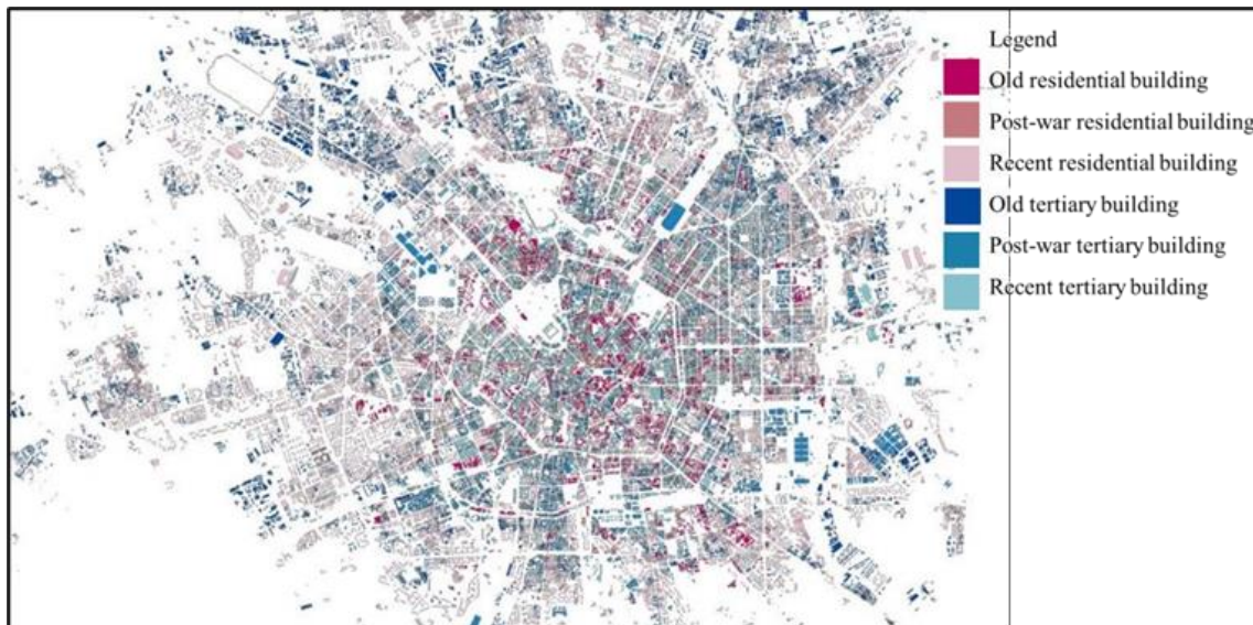
Figure 8. Buildings classification application at urban level for Milan city, as result of best ANN retrain.
