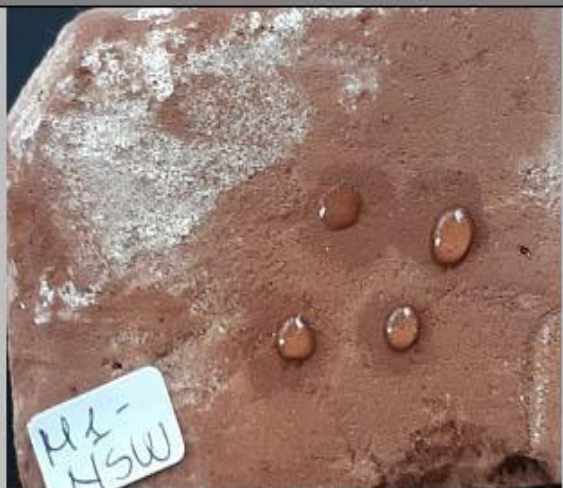
2- picture shows how the surface can absorb the droplets so fast
