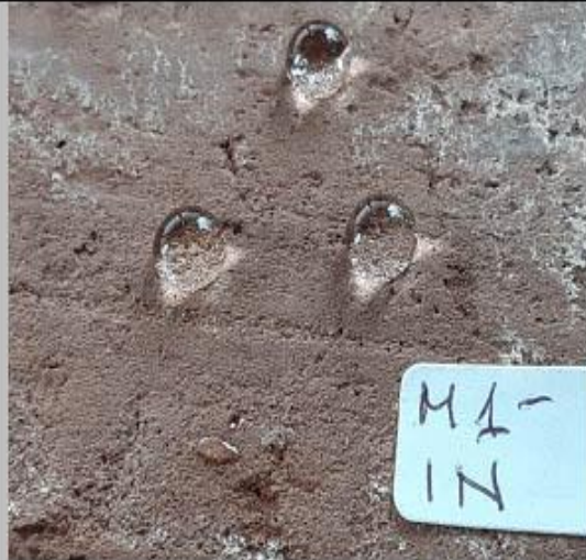
1-picture shows the droplets on the surface of the material and no color change
