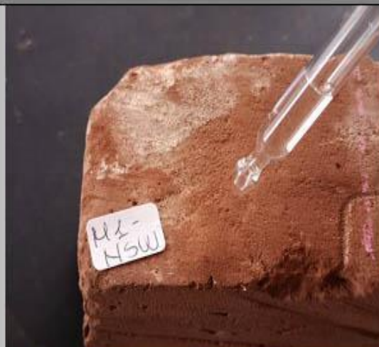
1-Picture shows the process of droplet test
