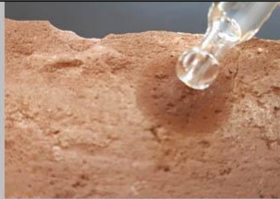
2 - Water Drop Test before the treatment: the water droplets are instantly absorbed from the material.
