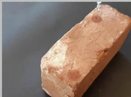
3- Water Drop Test before the treatment: the water droplets are instantly absorbed from the material.
