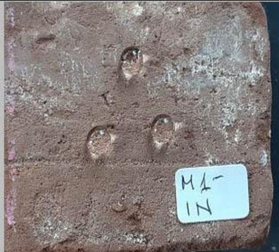
1-picture shows the droplets on the surface of the material and no color change
